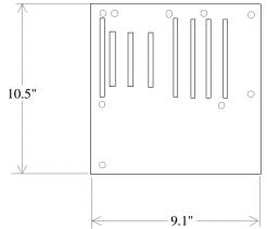
Figure 1. Classic/PCI i486 Baby-AT Motherboard dimensions.
